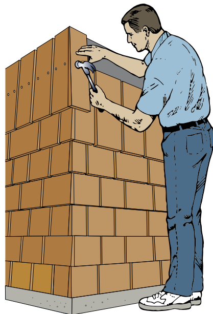
Figure 9: Fitting Laced Corner Courses
